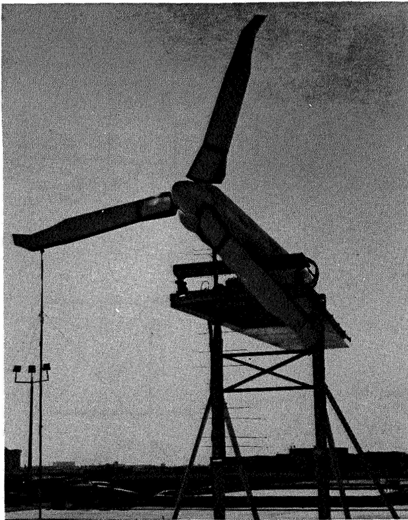
Figure 10. ATB rotor with swept-tapered tips and extended trailing edge cuffs.
