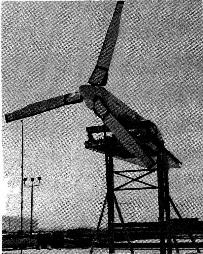
Figure 11. ATB rotor with square tips and extended trailing edge cuffs.
