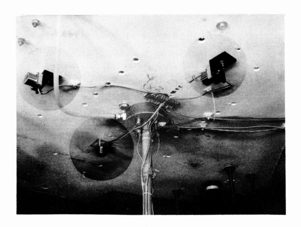
ORIGINAL PAGE IS OF POOR QUALITY The reflector-mounted rate sensor package, shown in the extreme left of the figure, senses three axis angular rates at the reflector end of the mast. This information is used for the vibration suppression control law.
