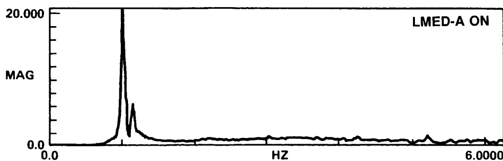
Figure 19. Magnitude of torque-Y to Acc-A transfer function in configuration 2; (open loop) LMEDA. Closed loop effects of LMED-A on Y-torquer to Acc-A transfer function.
