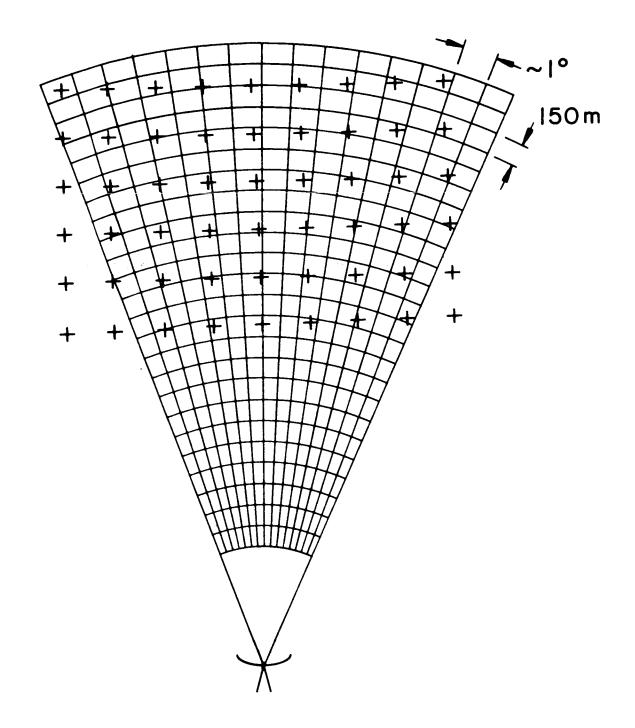
Figure 3. Two-dimensional schematic view (not to scale) of Doppler radar data overlaid by an orthogonal Cartesian grid.
