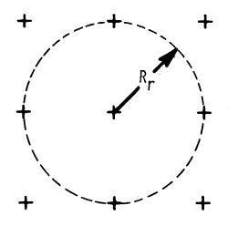
Figure 4. A close-up of the Cartesian grid point that is used in a Cressman objective analysis scheme.
