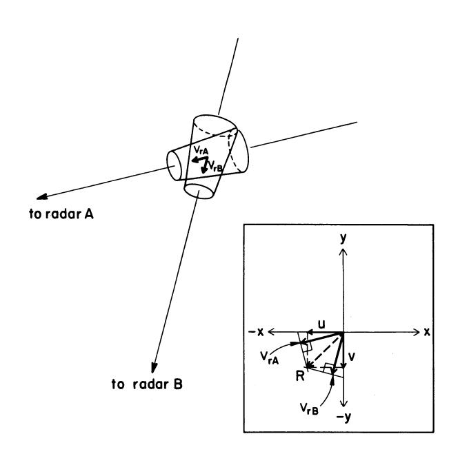
Figure 2. The resolution of  $V_{rA}$  and  $V_{rD}$  into orothogonal components. Inset shows graphical resolution of two non-orthogonal into two orthogonal components using direction cosines.
