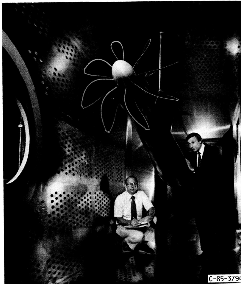
FIGURE 6. - THE SR-7A PROP-FAN INSTALLED IN THE NASA LEWIS 8- BY 6-FOOT WIND TUNNEL.
