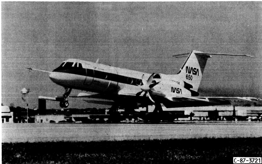
FIGURE 3. - LARGE SCALE VERSION OF THE SR-7A PROP-FAN ON THE GULFSTREAM II AIRPLANE.
