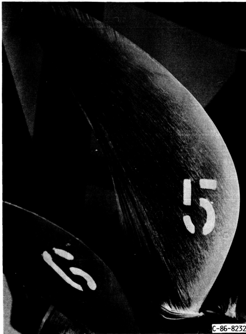
FIGURE 38. - FLUORESCENT OIL FLOW PATTERN ON THE 45^{\circ} SWEEP SR-3 PROP-FAN SUCTION SIDE SHOWING A SMALL LEADING EDGE VORTEX PATTERN AT MACH 0.60 HIGH POWER CONDITIONS. ( J = 3.17 , C_p = 2.14 , \beta_{0.75R} = 62.0^{\circ} .)
