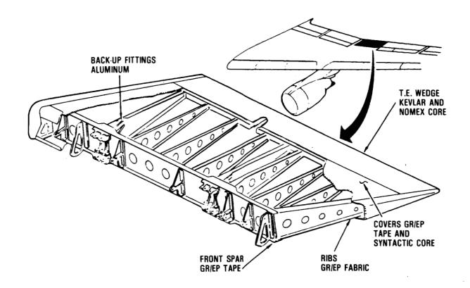
Figure 1. - Advanced Composite Aileron Assembly
