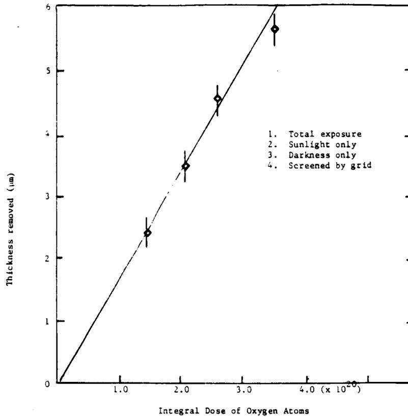
Figure 1. Vitreous Carbon Dosimeter, STS-8 Exposure
