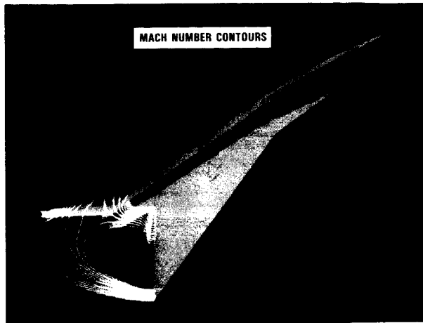
Figure 13. Wing Vortex Defined by Mach Contours
