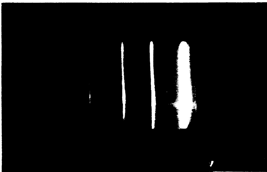
Figure 3: Arc Transition in a Negative Point-Plane Gap.
