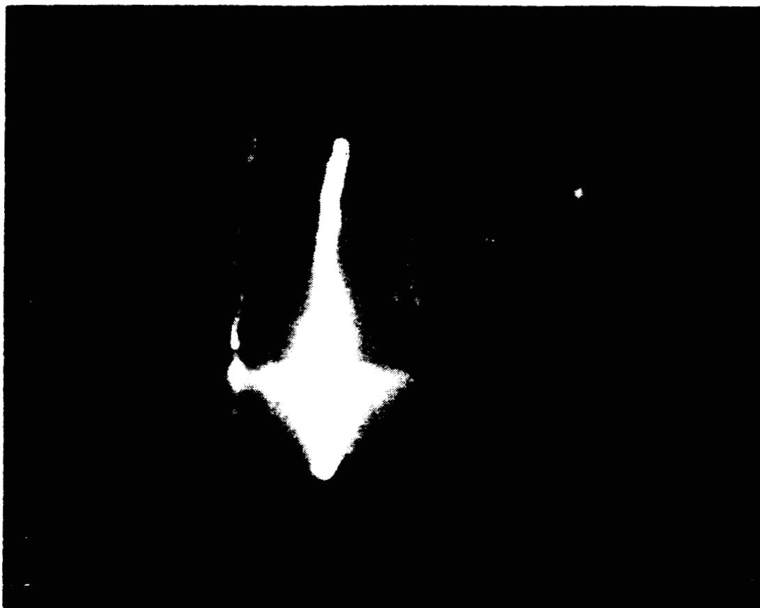
Figure 2: Leader Propagation and Arc Transition in a Positive Point-Plane Gap.
