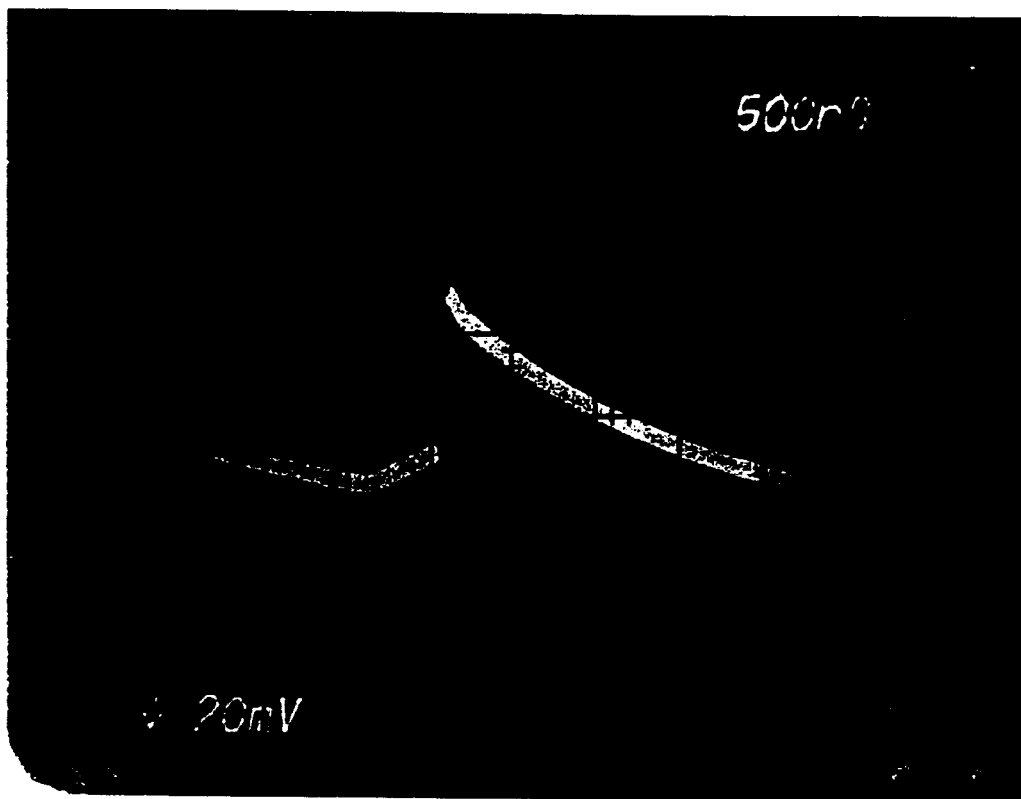
Figure 25: (Continued) (b) Transition to arc with leader propagation.
