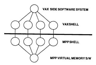
When the Parallel Pascal subroutine has completed its task, control is returned to the VAX via a call to a specially written MCL routine called HALT. Once control has been returned to the VAX, the applications program can interact with the user so that he can select the next function to be performed on the MPP.
