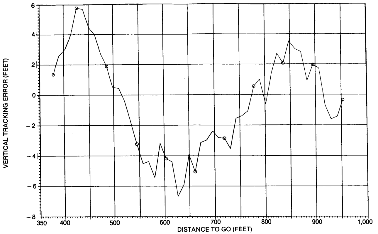
Figure 31. Vertical Tracking Error as a Function of Distance to Go (Case 8)
