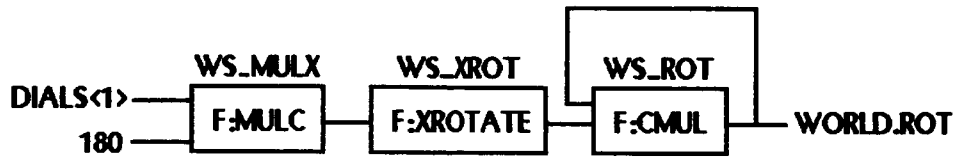
Fig. 2. Schematic of rotation function network
