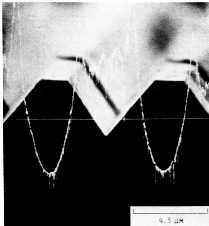
FIGURE 10. - ELECTRON BEAM INDUCED CURRENT SUPERIMPOSED ON THE V-GROOVE STRUCTURE AT THE POSITION NOTED BY THE HORIZONTAL LINE.
