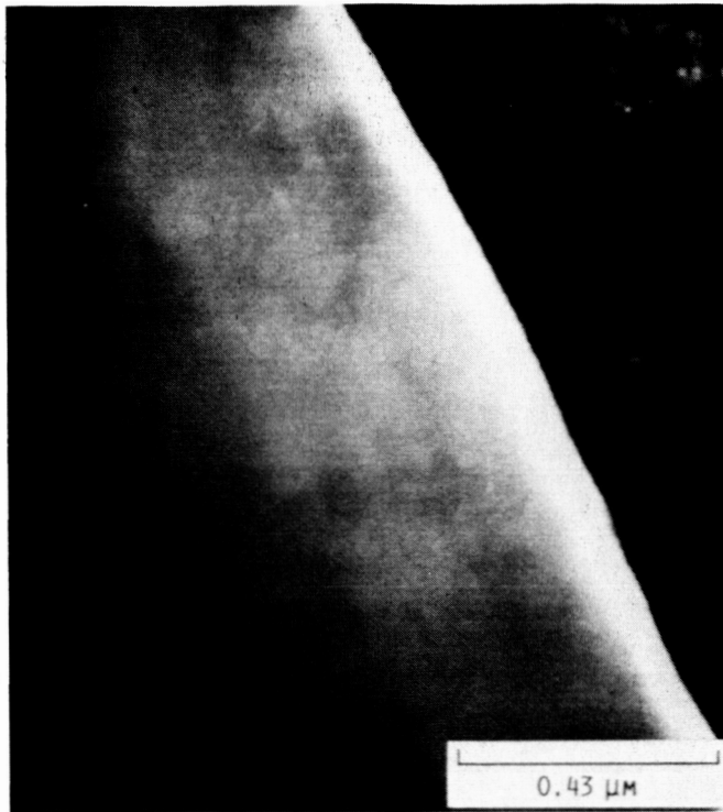
FIGURE 9. - HIGH MAGNIFICATION SEM MICROGRAPH SHOWING PORTION OF V-GROOVE WITH EPILAYERS.
