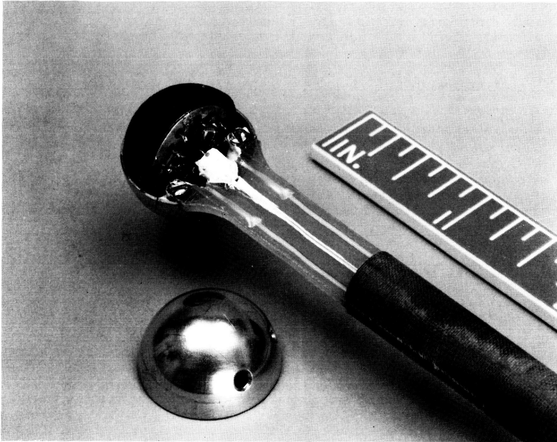
Figure 2-7. Photograph of the ac probe with one hemisphere removed
