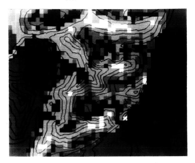
Figure 5. Model of organic carbon mapped by TM ratios 1/4, 3/4 and 5/4 superimposed on 20 ft contour lines of a bare soil field. The content of organic carbon in g/kg is 5.0, white; 9.0, yellow; 12.2, pink; 16.0, orange and 21.0, dark red. Plant cover is coded green.
