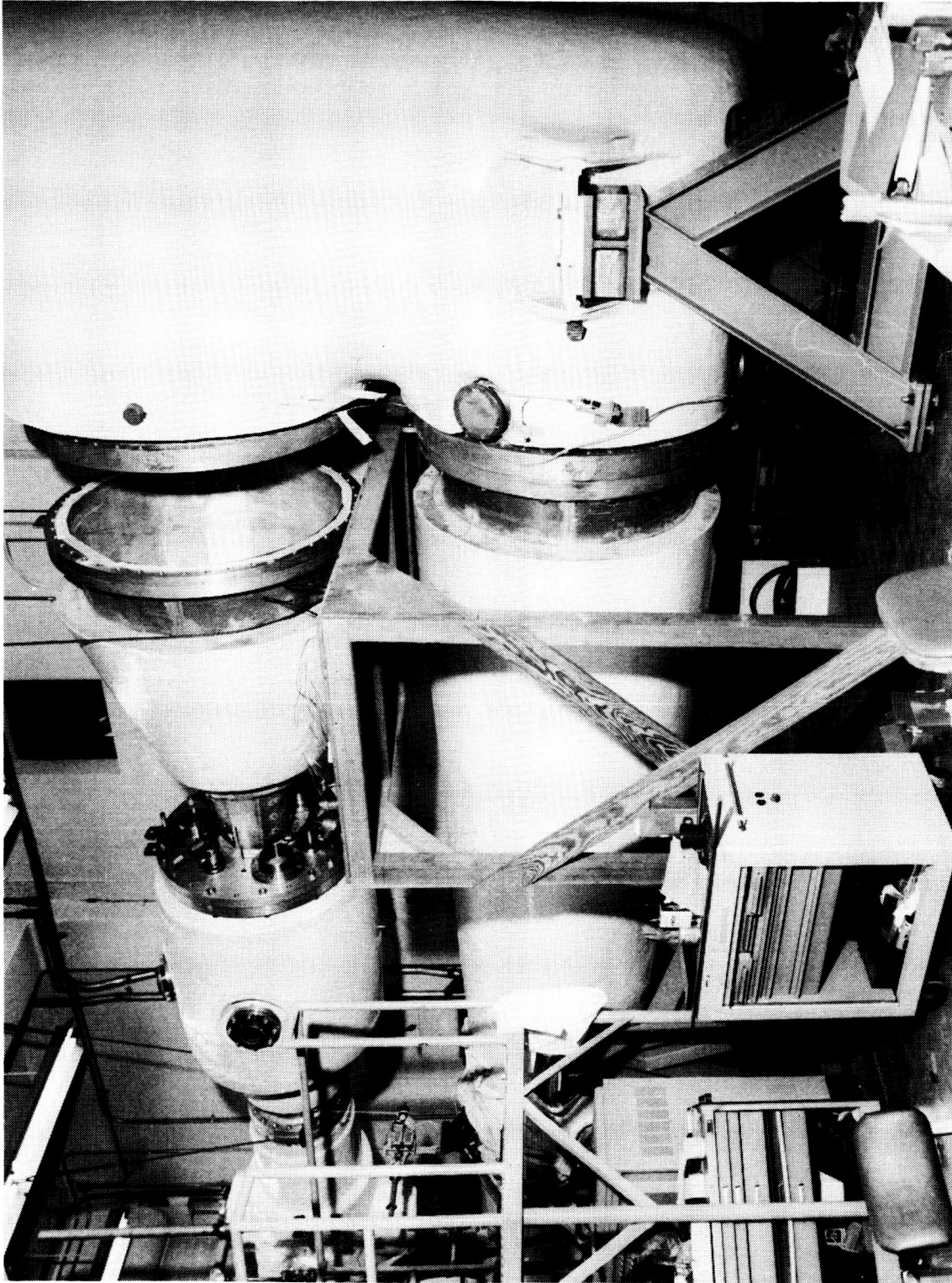
Figure 2.- The Langley 0.3-m TCT with three-dimensional test section during initial assembly.
