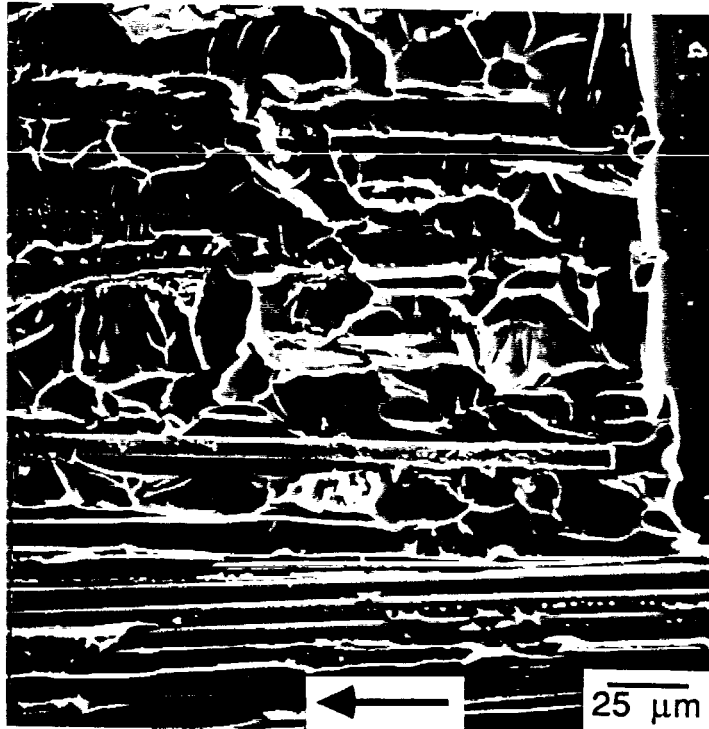
Fig. 6. Sem photograph of the fracture surface of the DCB specimen JS120-2 (control). Large pockets of deformed material on the fracture surface are a result of voids which have grown very large during fracture.
