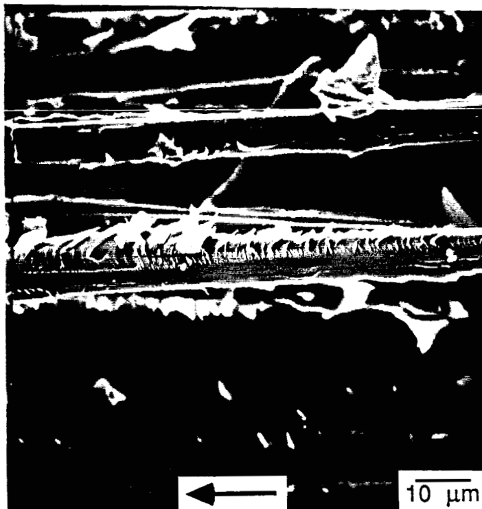
Fig. 8. SEM photomicrograph of the fracture surface of the DCB specimen JS120-2 (control). Excellent adhesion of the resin to the fibers is apparent.
