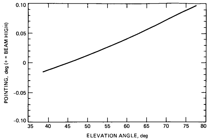
Fig. 4. Beam pointing vs elevation angle with subreflector y and z focusing
