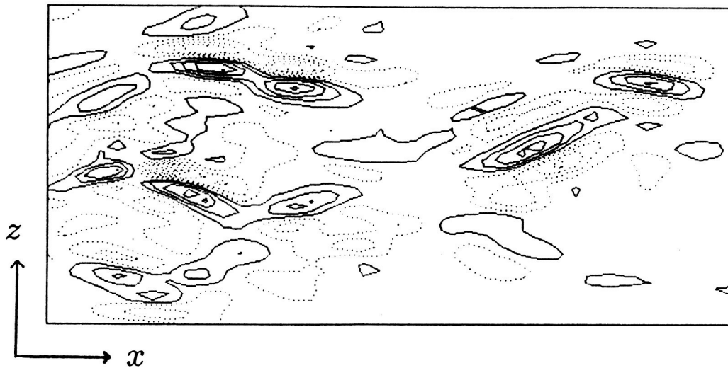
Figure 8. Normal-velocity contours. y^+ \approx 0.03 . — positive, v^+ = 0.002, 0.006, 0.01 ; \cdots negative, v^+ = -0.002, -0.006, -0.01 .
