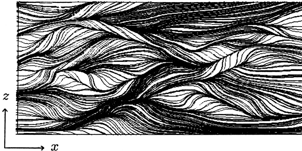
Figure 7. Skin-friction lines. The flow is from left to right.
