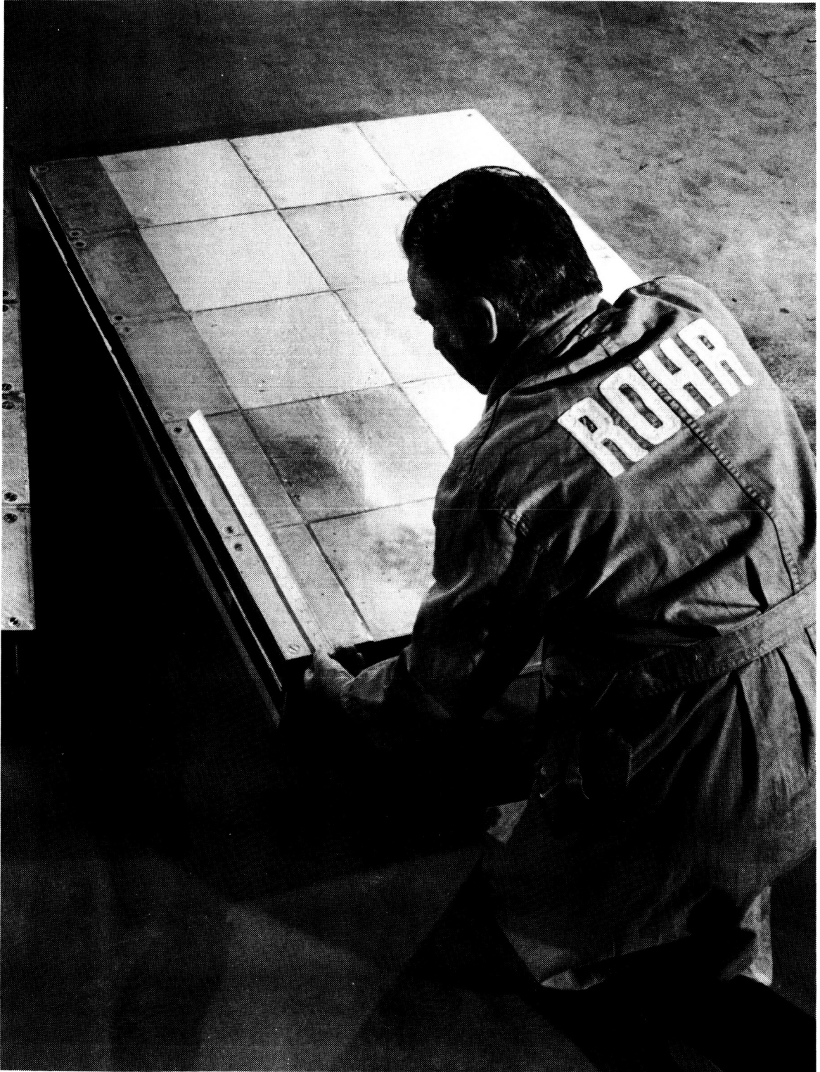
Figure 17. Superalloy--Titanium--Silica Sandwich Panel--20-Panel Array
