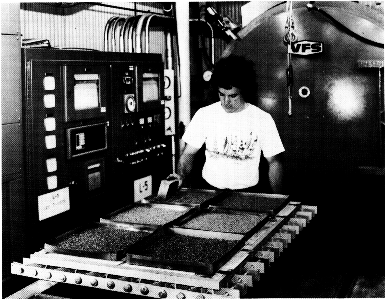
Figure 19. Six Titanium Subassemblies being Removed from Vacuum Furnace after LID Bonding
