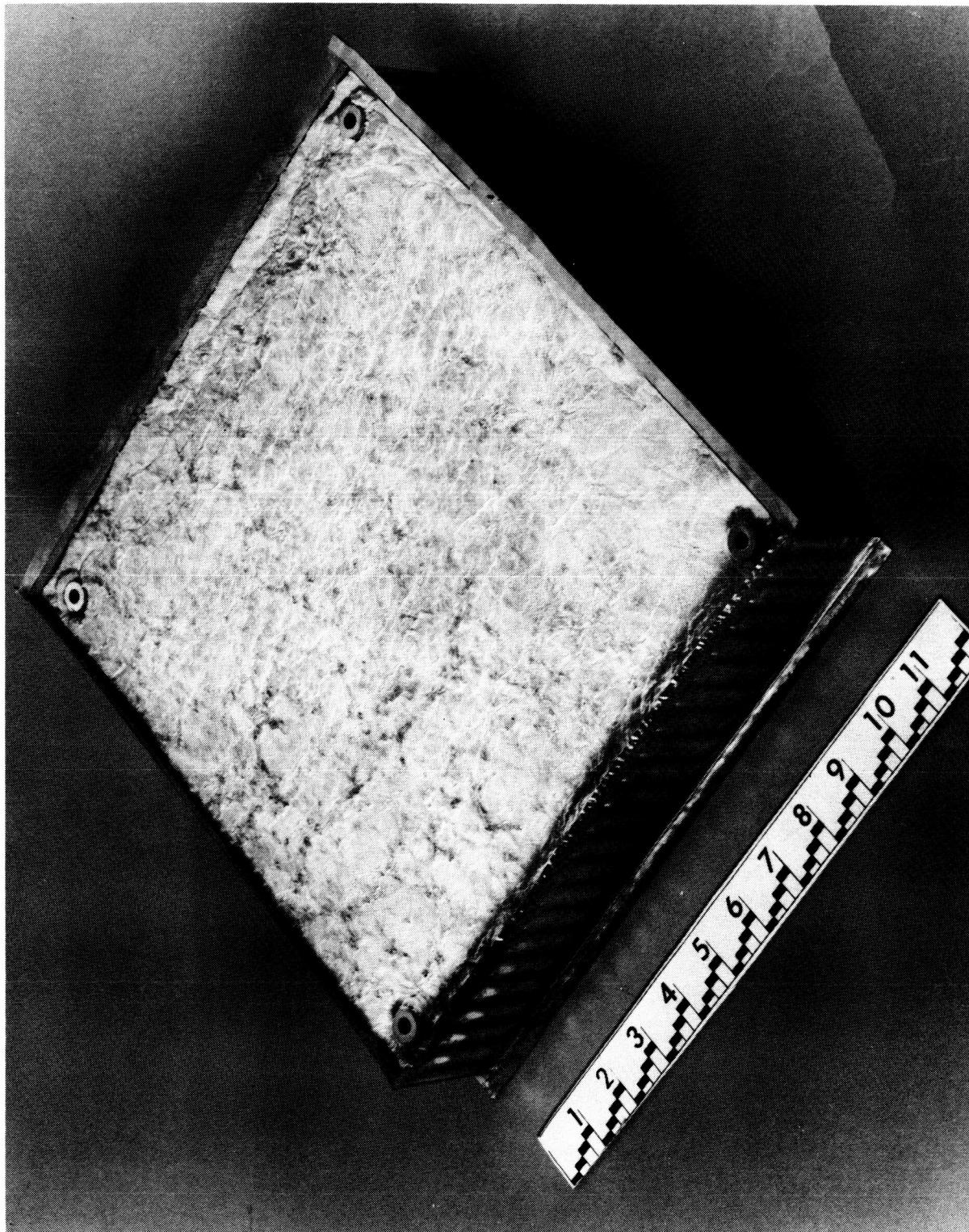
Figure 13. INCONEL 617 Subassembly with DYNAFLEX and Q-FIBER FELT Installed
