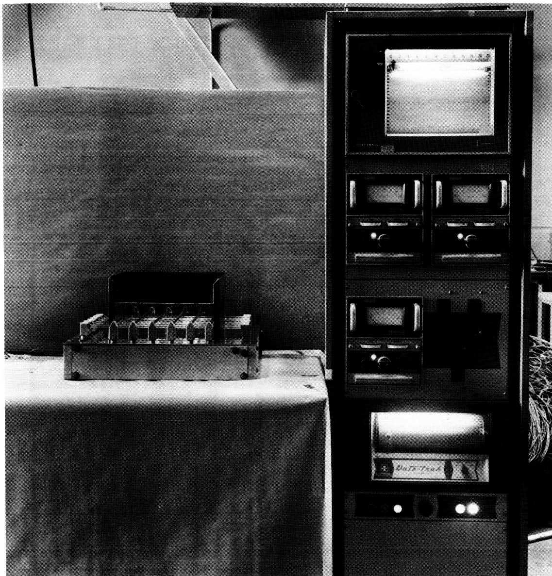
Figure 26. Guarded Hot Plate with Thermac Controller
