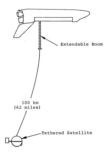
Figure 1: Tethered Satellite Experiment
