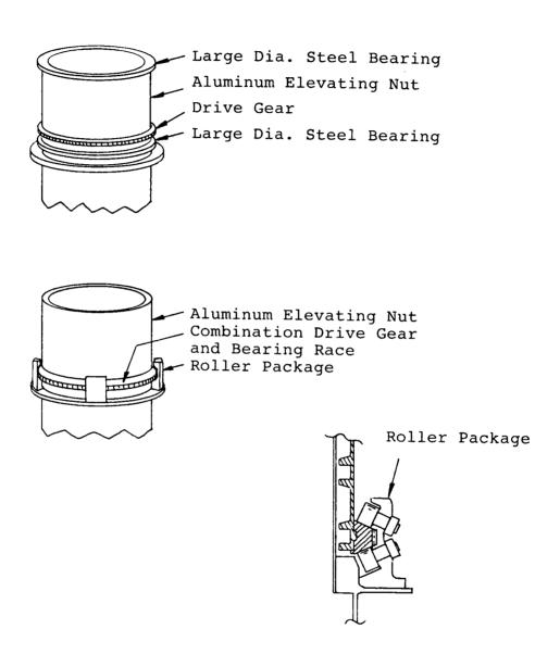
Figure 7: Bearing Comparison
