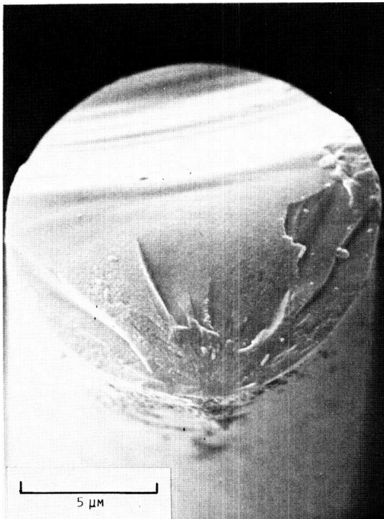
(B) FIBERS TREATED AT 1 ATM AR, WITH WT LOSS OF 0.8% AND TENSILE STRENGTH OF 235 KSI (1620 MPa).
