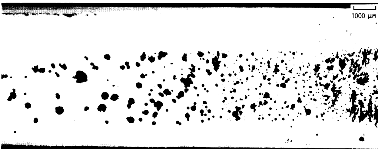
(B) ATOMIZING AIR PRESSURE, 450 kPa. DROPLET DIAMETER = 12.0 μm; WATER PRESSURE - 535 kPa.
