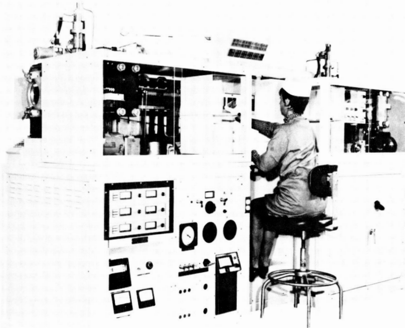
FRONT VIEW: OPERATOR LOADS AND UNLOADS SUBSTRATES
