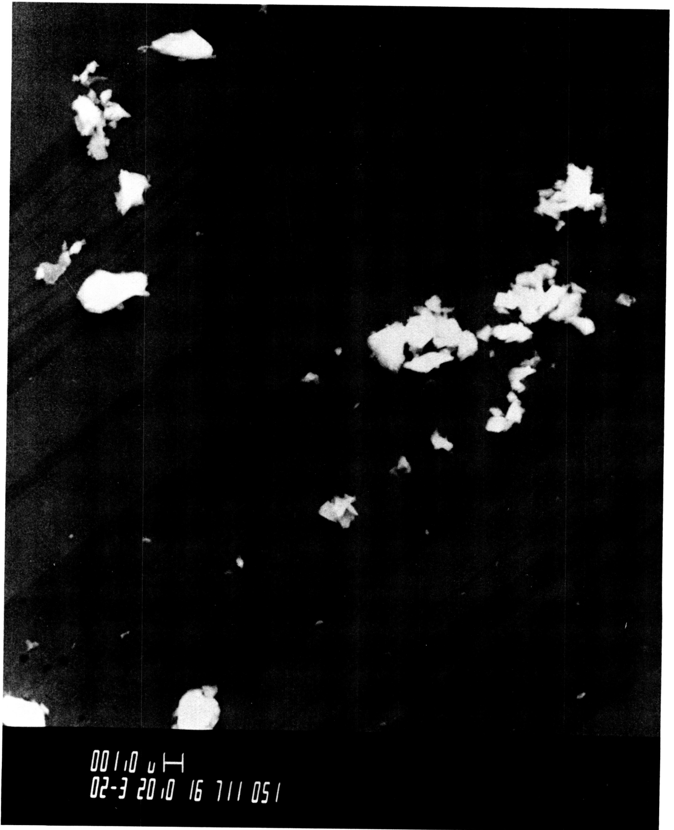
Figure 8a. 2000x SEM photomicrograph of a test coupon artificially contaminated to 6000 particles/cm 2 with 0.1-5 \mu m A/C test dust particles in methyl ethyl ketone.
