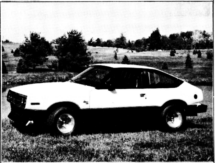
Upgraded Mod I AMC Spirit Combined Mileage Acceleration* 1984 10.7 km/L (25 mi/gal) 25 s 1985 12.2 km/L (28.5 mi/gal) 16 s
