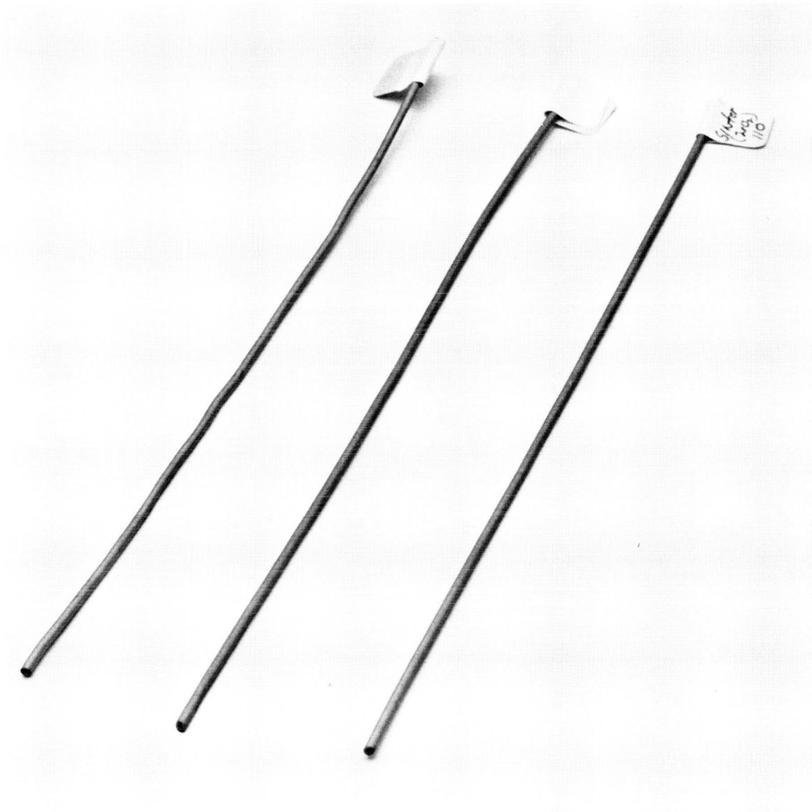
Figure 7.- Samples of the type B die set sintered tubes, left to right, rhenium with 0%. 0.5% and 1.0% added stabilized zirconia.
