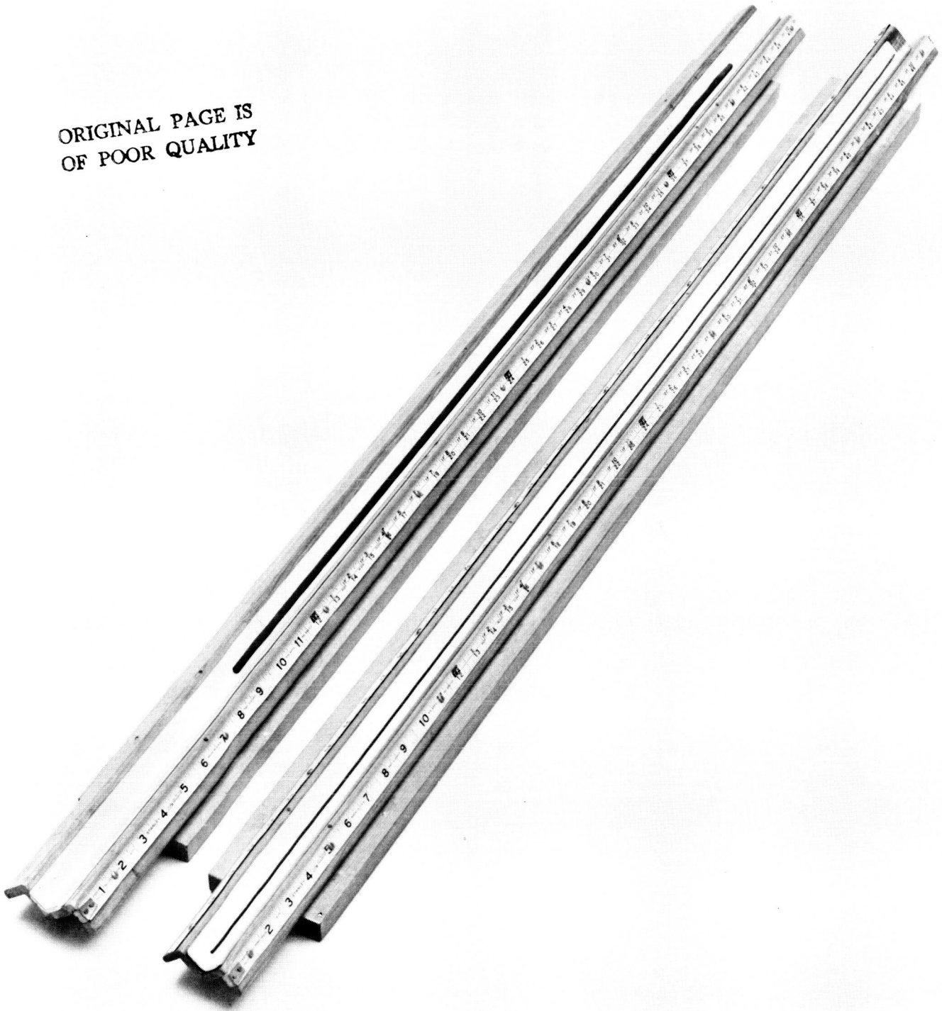
Figure 1.- Extruded straight green rhenium tubing with zirconia additives. Type A and Type B.
