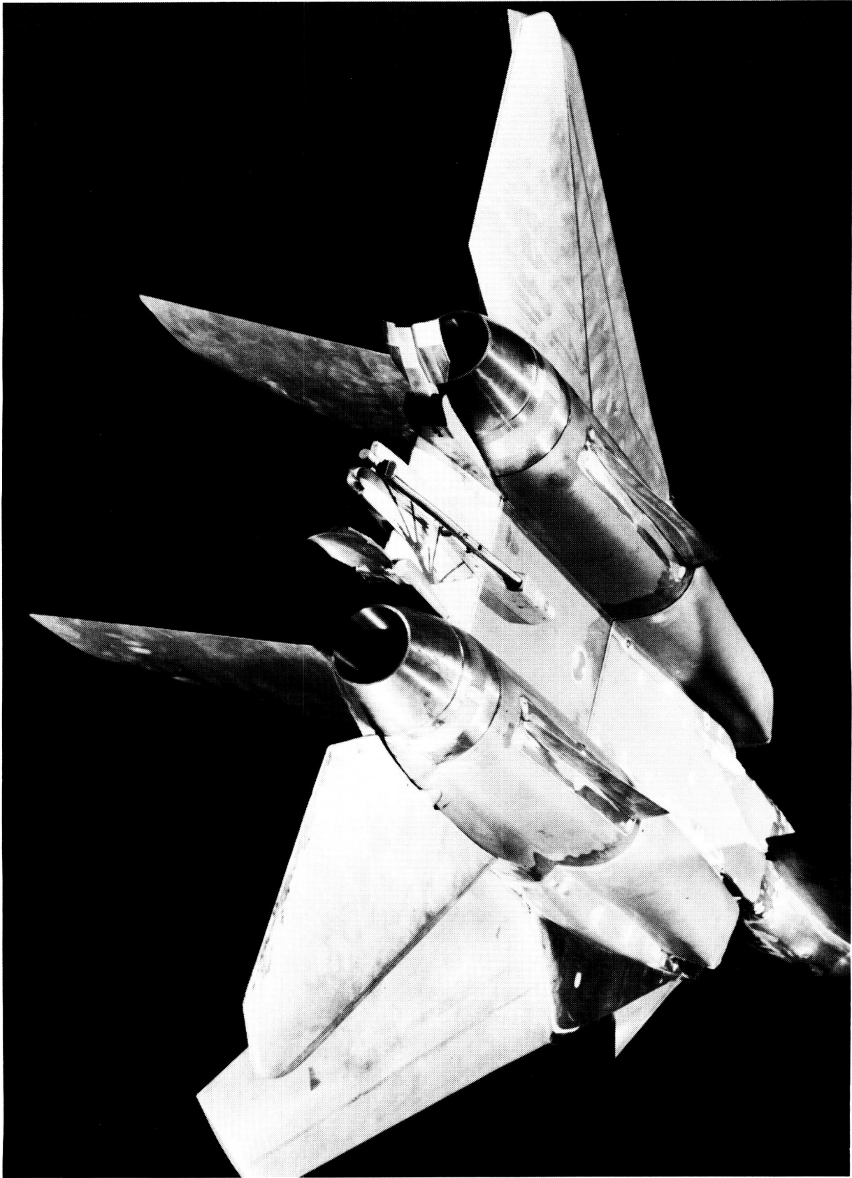
(c) Lower rear view showing F110 cruise nozzles and yaw vanes. Right vane deflected 20°.
