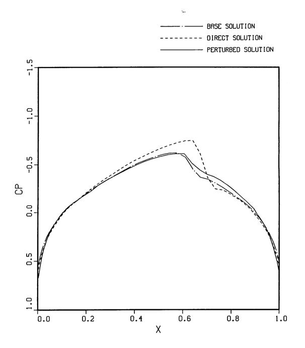
Figure 11.- Finite difference Solution with Coordinate Straining (11% biconvex airfoil).
