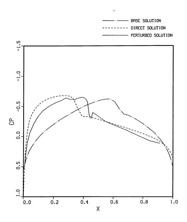
Figure 6.- Pressure Distribution Around a NACA0010 Airfoil,  $M_{\infty} = 0.808$
