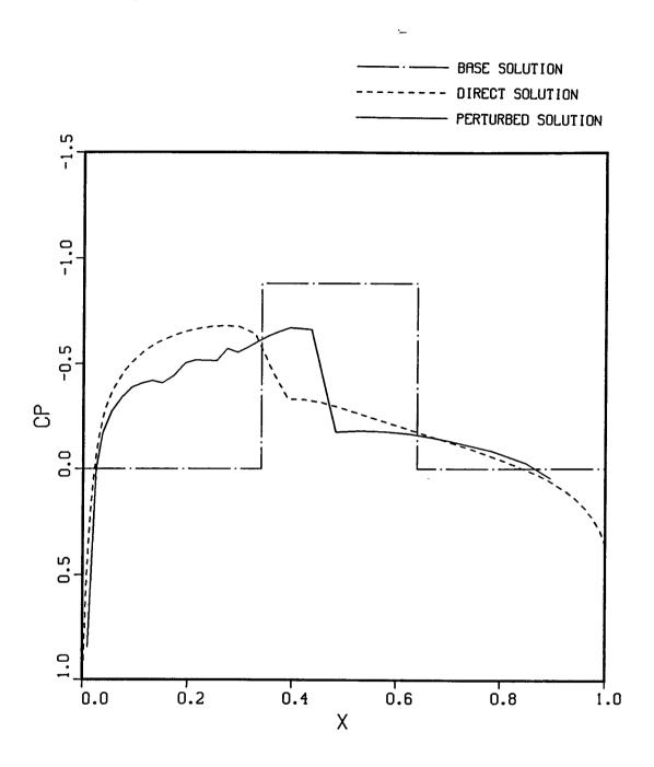
Figure 14.- Solution of Linear Constant Coefficient Equation (NACA 0010 Airfoil).
