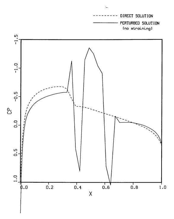
Figure 12.- Finite Difference Solution with Central Differences (NACA 0010 airfoil).
