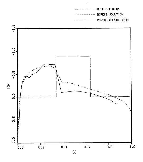
Figure 15.- Solution of Linear Constant Coefficient Equation with Modified Straining Terms (NACA 0010 Airfoil).
