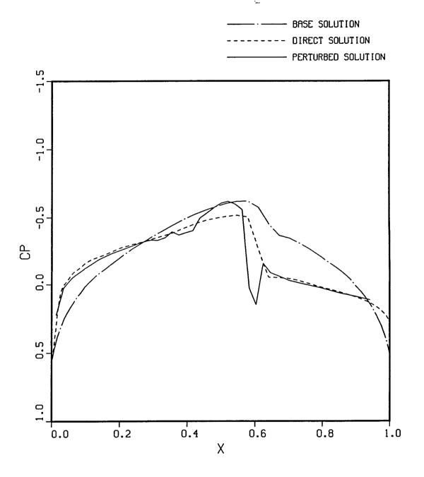
Figure 7.- Pressure Distribution Around a NACA 64A006 Airfoil,  $M_{\infty} = 0.875$
