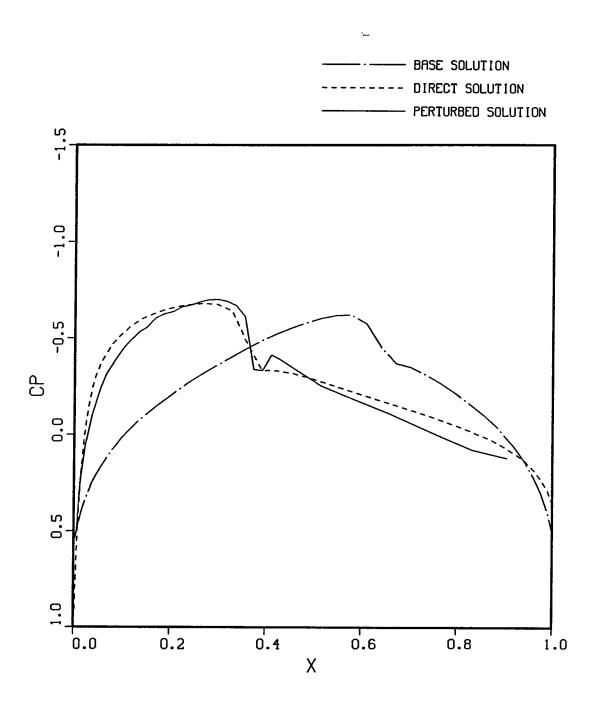
Figure 8.- Pressure Distribution Around a NACA 0010 Airfoil;  $M_{\infty} = 0.808$  with Double Straining.
