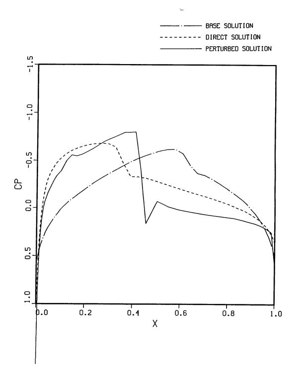
Figure 13.- Finite Difference Solution with Coordinate Straining (NACA 0010 Airfoil).
