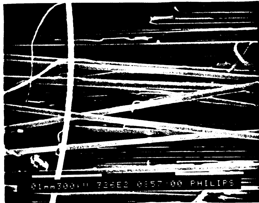
Figure 4.41 Scanning electron micrographs of virgin DCB specimen at end of crack. The top figure is at 163X, the bottom figure at 326X.
