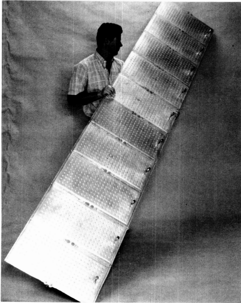
Figure 6-2 Aluminum prototype panel - dimpled surface.
