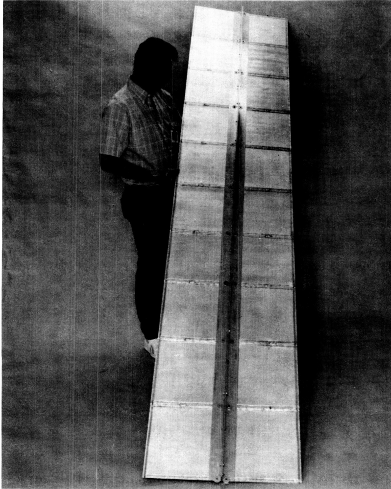
Figure 6-1 Aluminum prototype panel with "T" beam.
