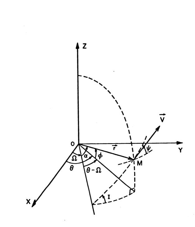
Fig. 2. Osculating Plane and Orbital Elements
