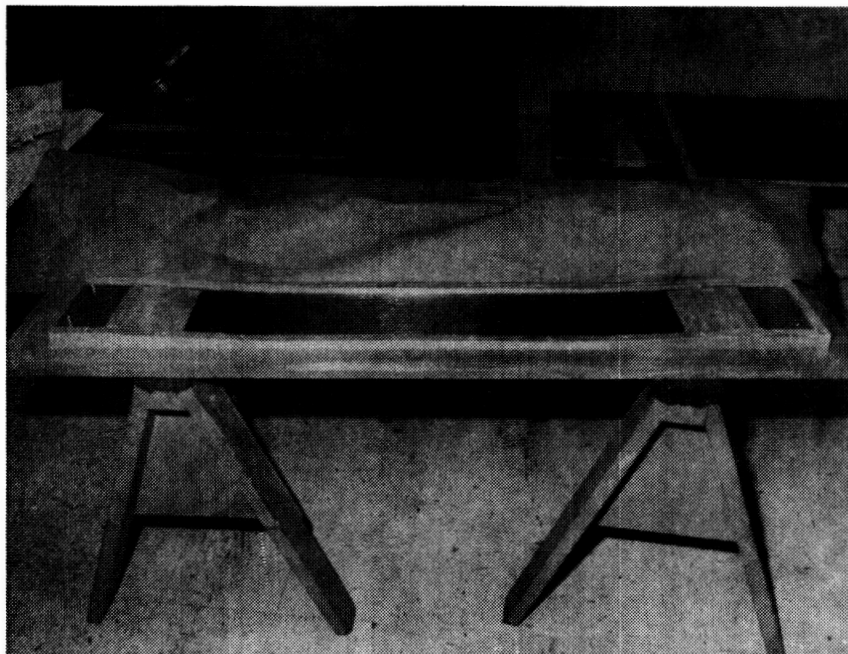
Figure 18. Overall View of Skin Tool with Completed Skin Layup
