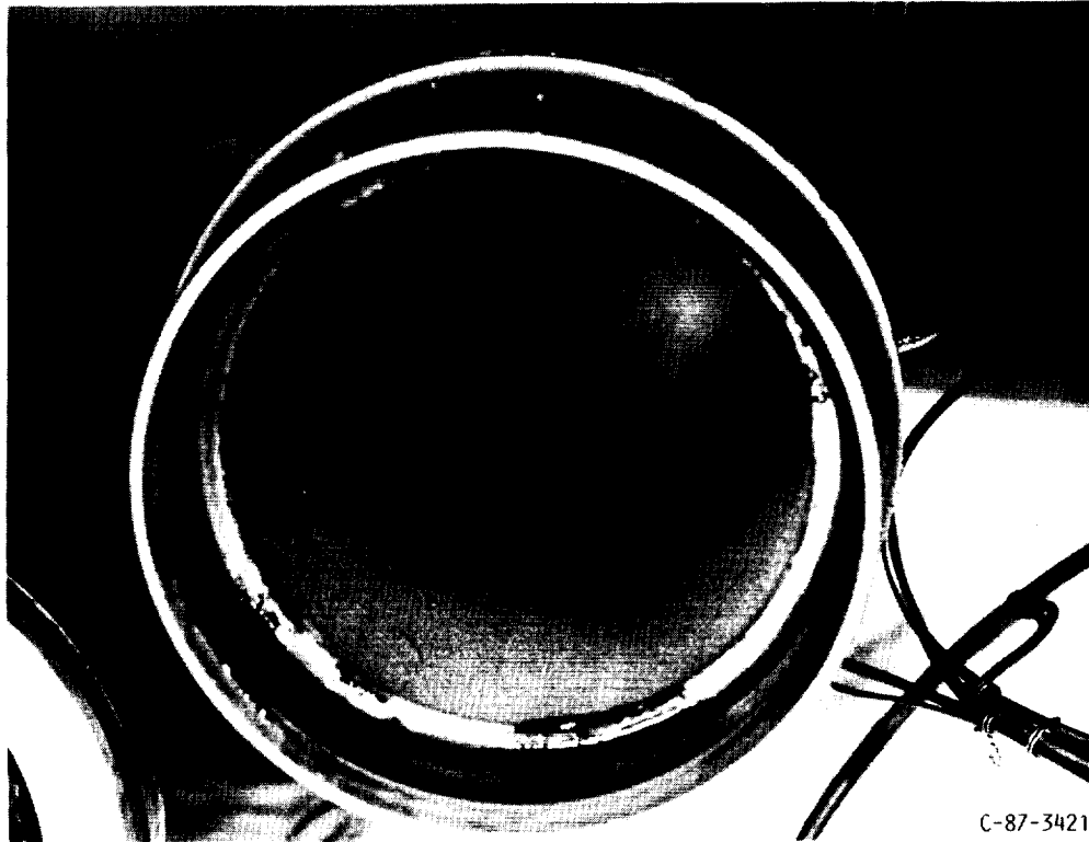
FIGURE 12. - PS200 COATING ON STIRLING ENGINE CYLINDER AFTER 22-HOUR ENGINE TEST WITH "HOT RINGS".
