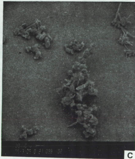
Figure 15.--SEM photomicrographs of as-received GTE SN502 \text{Si}_3\text{N}_4 powder.
