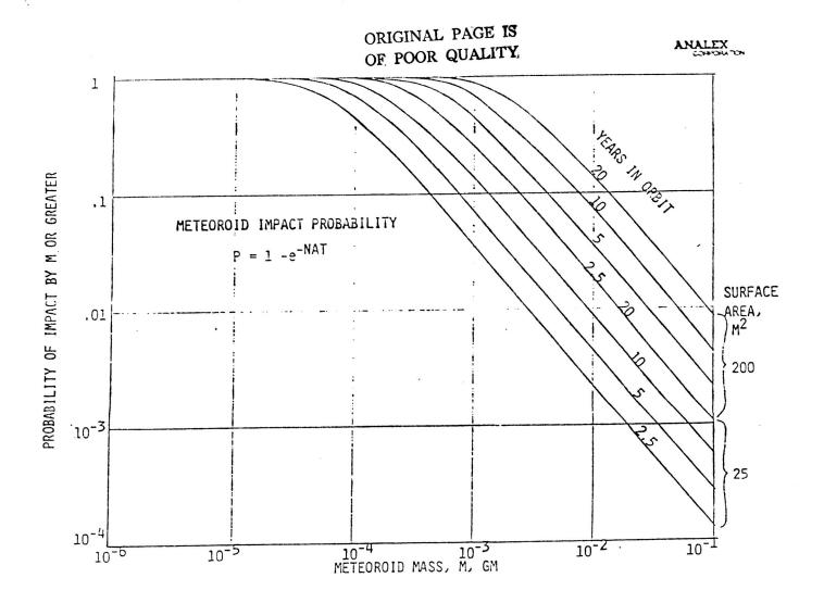
The hypervelocity impact probability was calculated from queueing theory for a stream of random events in which the probability of at least one event occurring in time T is given by l-e -NAT. This equation is based on a Poisson process of a steam of random events like calls coming in on a telephone line, or particles monitored by a Geiger counter, or cars pulling up to a gas station. Each event is just like the previous one, and there are no after effects on the occurrence of the next event.
