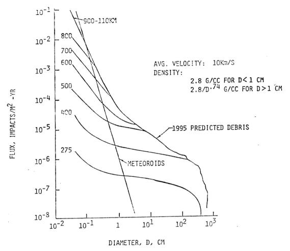
The predicted flux of orbital debris by the year 1995 is shown in this slide. The population of small debris is kept down by atmospheric drag at the lower altitudes. At space station altitudes, the flux of debris smaller than 1cm is lower than meteoroid flux. As the debris size increases, the flux rate decreases but more slowly than meteoroids so that above 1cm, the debris-flux is higher.
