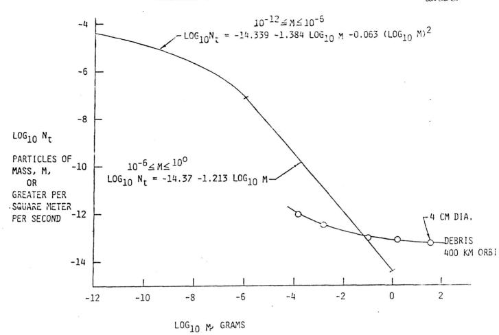
This slide shows the debris flux-mass model at 400 km superimposed on the meteoroid model. The cross-overpoint occurs at a mass of about 0.1 gm. Because of the differences in average density, 0.1 gm meteoroid is a sphere about 4mm dia. A typical debris of the same mass is 2mm dia.; about the size of a B.B. shot.
