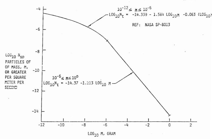
This shows the average flux-mass model used for the study. It is for a distance in space of 1 A.U. For much larger distances, a gravitational defocusing factor can be applied which tend to reduce the flux values.
