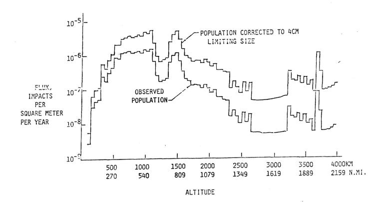
This shows the debris population as a function of altitude. The lower curve is based on the observed population. The upper curve is corrected for the fact that the tracking limit is 4cm and hence includes the unobserved population. At a space station altitude of around 400 km, the total population is believed to be about 2-1/2 times the observable population.
