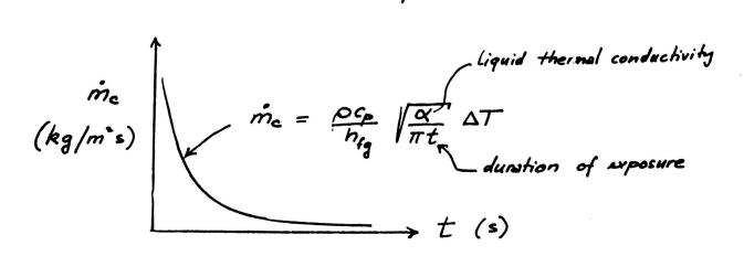
Condensation on turbulent liquid :
