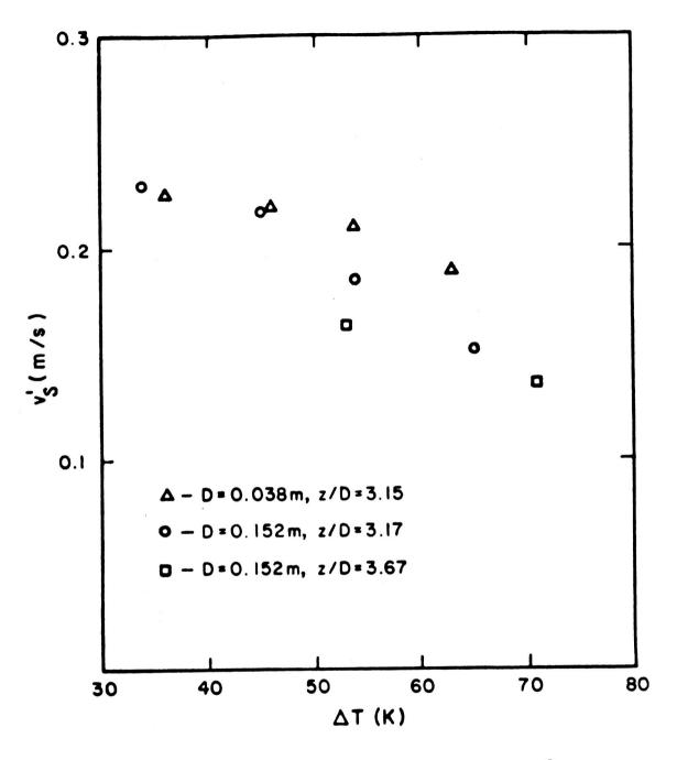
Threshold turbulence level for onset of condensation bursts
