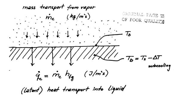
Condensation on static liquid:
