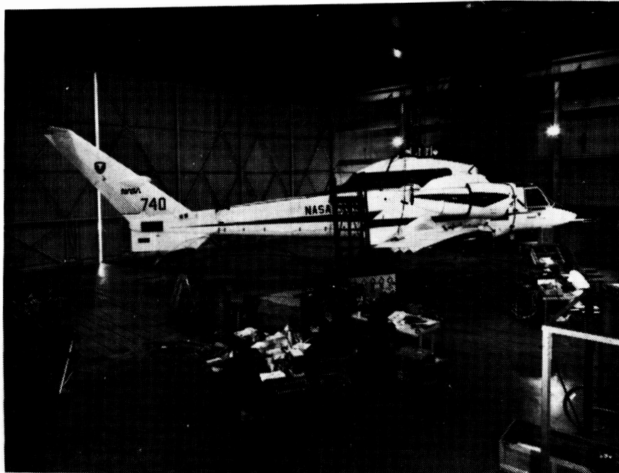
FIGURE 45. RSRA shake test setup.
