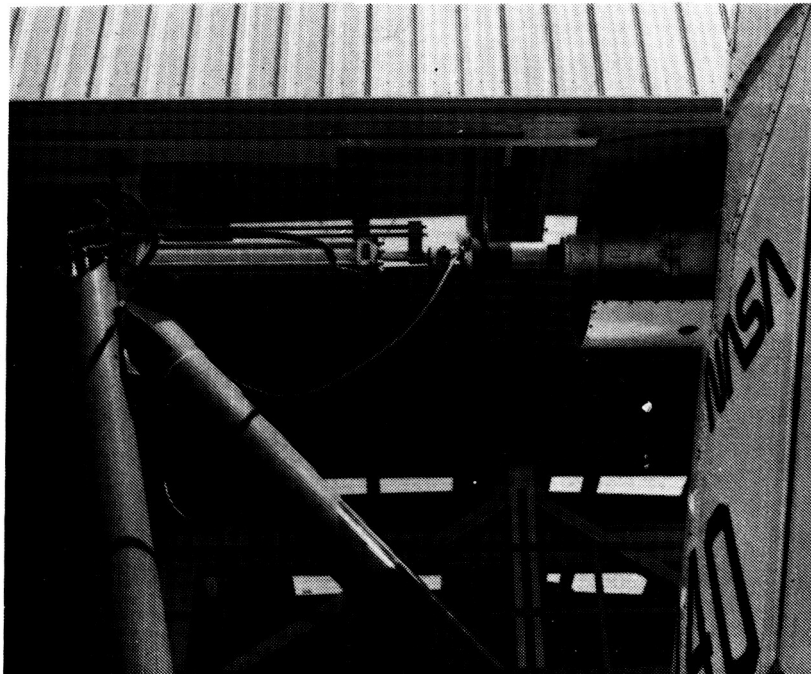
FIGURE 42. RSRA load measurement system calibration facility.
