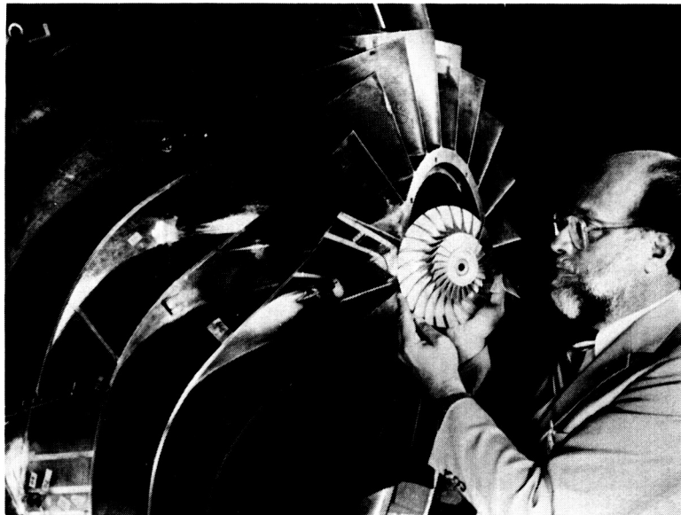
FIGURE 8. - LARGE LOW-SPEED CENTRIFUGAL COMPRESSOR NEW FLOW PHYSICS AND CODE VALIDATION RIG.
