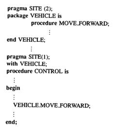
Our translation system would replace the local call to the procedure VEHICLE.MOVE\_FORWARD with the appropriate remote call. Similarly any references in CONTROL to data objects defined in package VEHICLE would be translated into appropriate remote references as would task entry calls. Note that the user need only use the normal procedure call mechanism to cause the vehicle to move.
