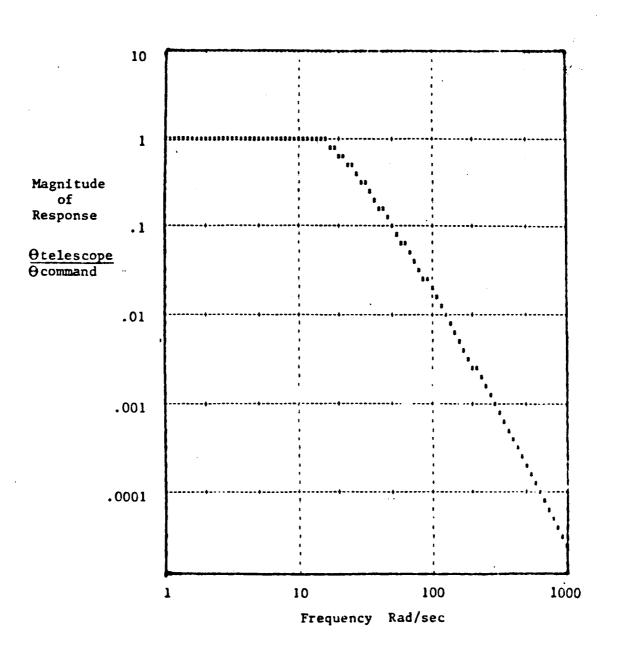
Figure 2-3. Fine-Pointing Control System Response to a Sinusoidal Command Signal
