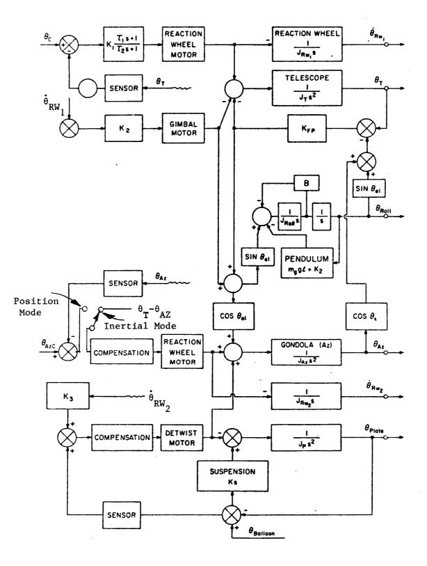
Figure 2-5. Block Diagram of Azimuth and Cross-Elevation Servos
