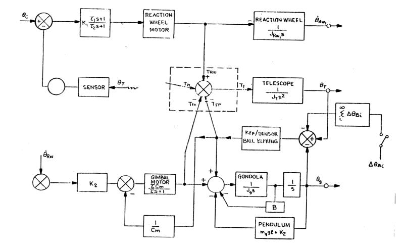
Figure 2-2. Nonlinear System Block Diagram
