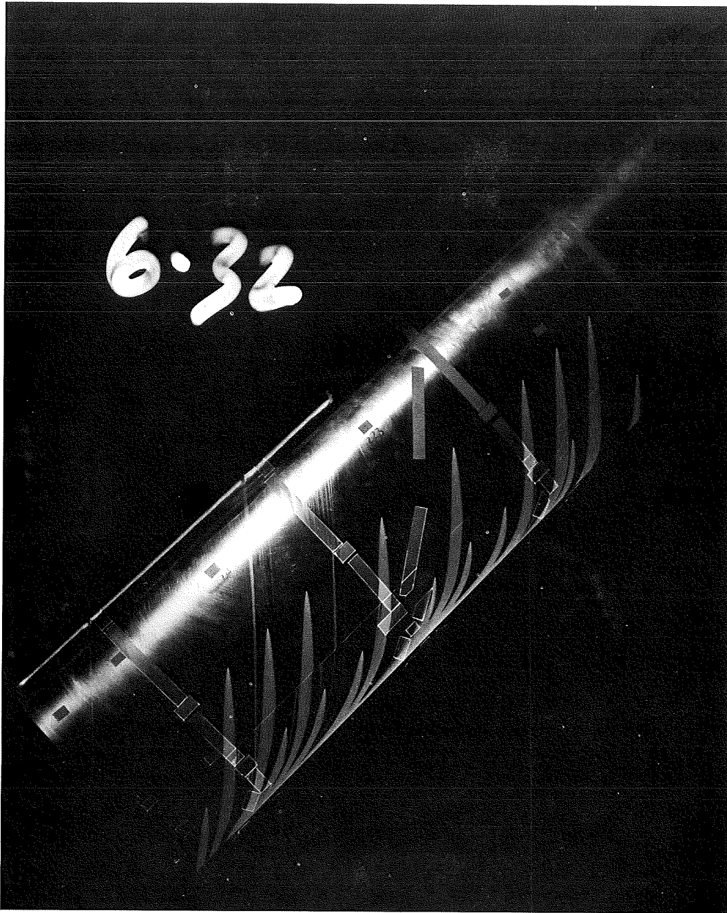
Figure 10.- Oil-flow photograph of upper-surface flow pattern at \alpha = 5^\circ , M = 0.70 , pressure ratio of 2.0.
