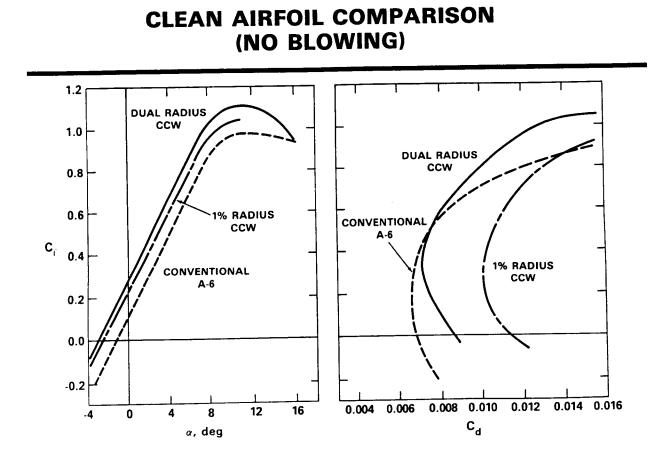
IX. The mechanical system required to rotate the dual radius circulation control flap would be equivalent to the system required for a simple single slotted Fowler flap. The undeflected dual radius circulation control flap would have no significant impact on cruise performance. The dual radius flap provides a means of mechanically varying the wing chamber independent of the circulation control blowing.
