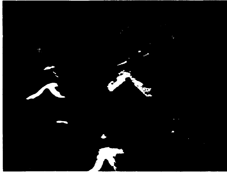
Figure 4.54: Decanted interface. Growth rate: 3.68 cm/hr with 200 rpm spin-up/spin-down. Magnification: 2.07 kX.
