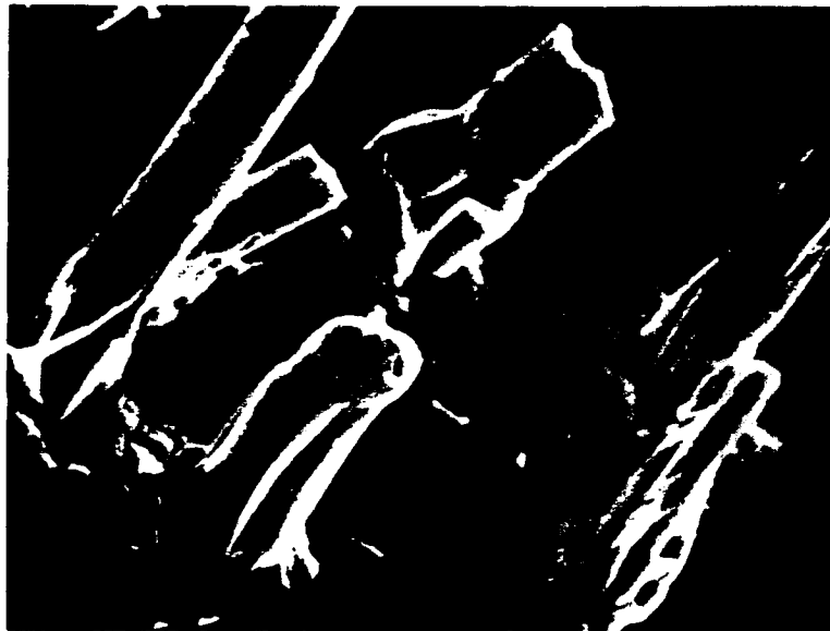
Figure 4.10: Fracture surface. Growth rate: 1.05 cm/hr, Growth direction: left to right. Magnification: 5.1 kX
