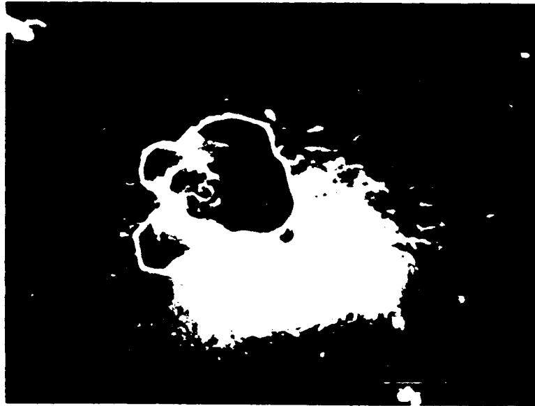
Figure 4.34: Decanted interface. Growth rate: 0.4 cm/hr with 100 rpm spin-up/spin-down. Magnification: 2.12 kX.
