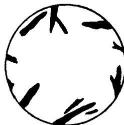
Figure 4.62: Microstructure of MnBi-Bi eutectic solidified at 0.25 cm/hr with 100 rpm spin-up/spin-down and run 3.
