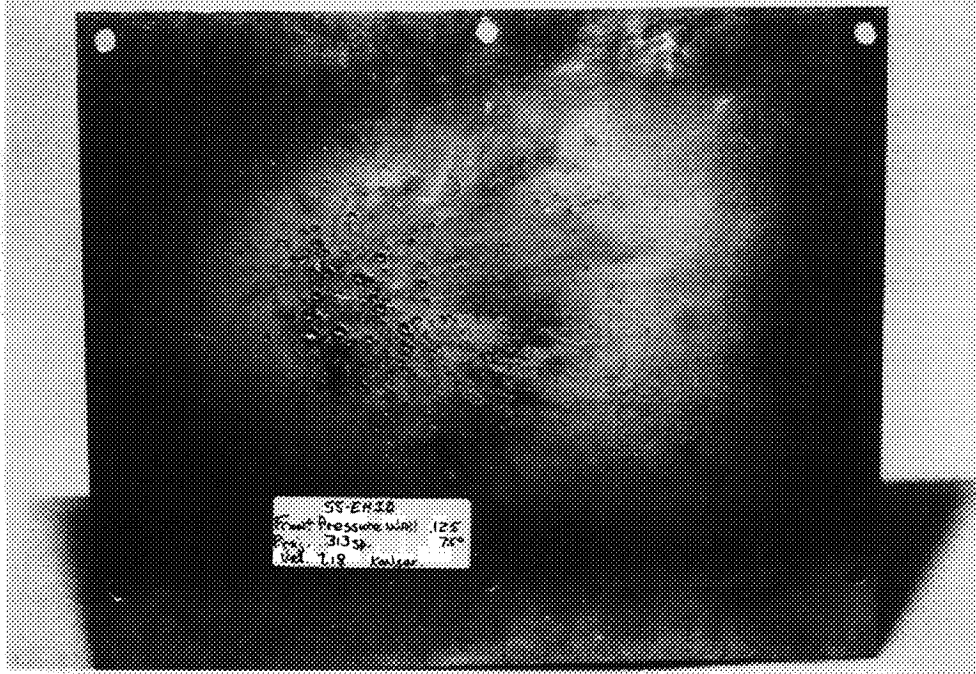
Figure 5b. 75-deg impact (EH1D), pressure wall plate.
