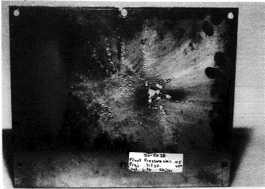
Figure 3b. 45-deg impact (EH1B), pressure wall plate.
