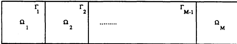
FIG.2.1 Decomposition by aligned subdomains
