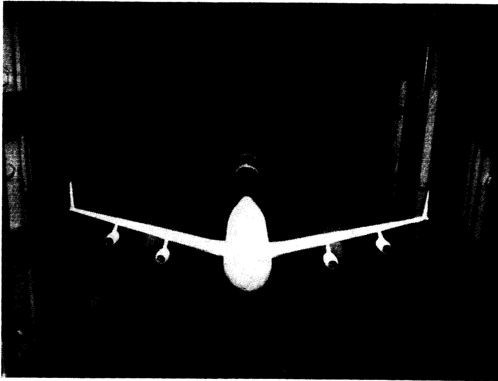
Figure 7. Wind-tunnel high-speed model.
