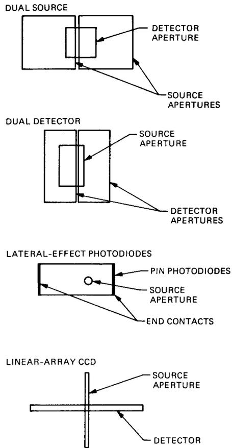
**Fig. 6. Non-scanning detection schemes used in commercial autocollimator**
