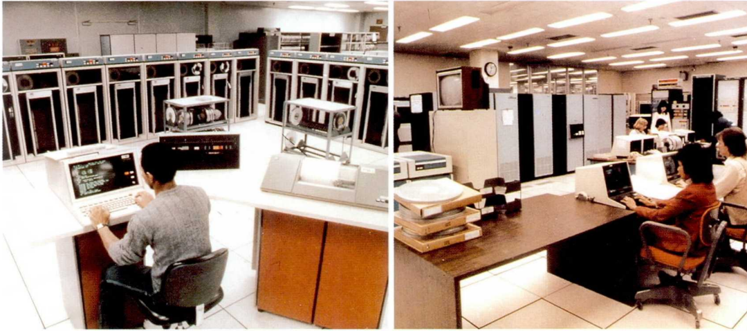
Figure 113. Two views of the Spacelab Data Processing Facility at Goddard Space Flight Center. The Spacelab output processing system (SOPS) is shown on the left; the Spacelab input processing system (SIPS) is on the right.
