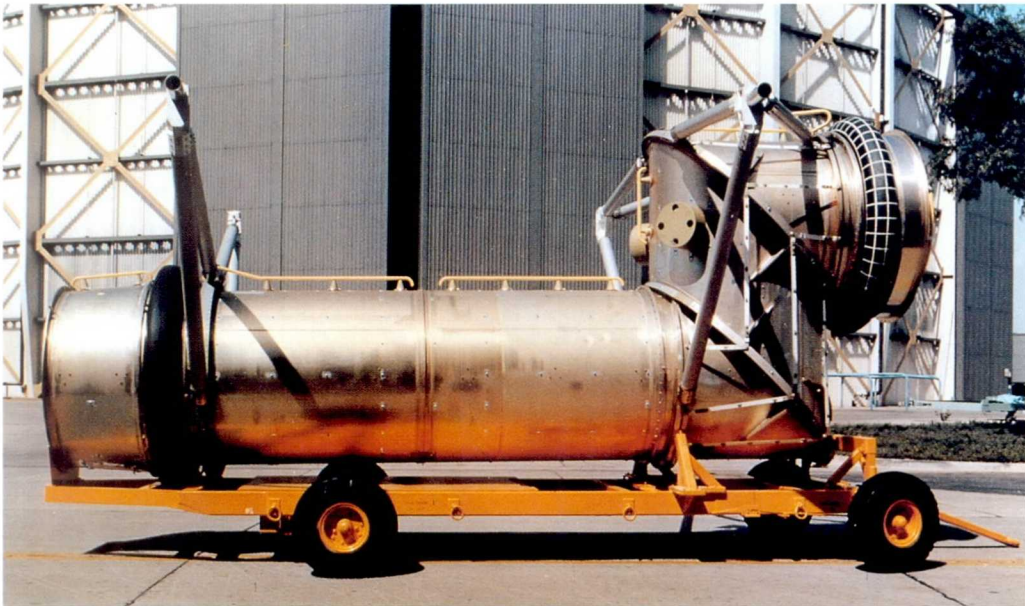
Figure 80. Completed transfer tunnel unit at the McDonnell Douglas facility in Huntington Beach, California.
