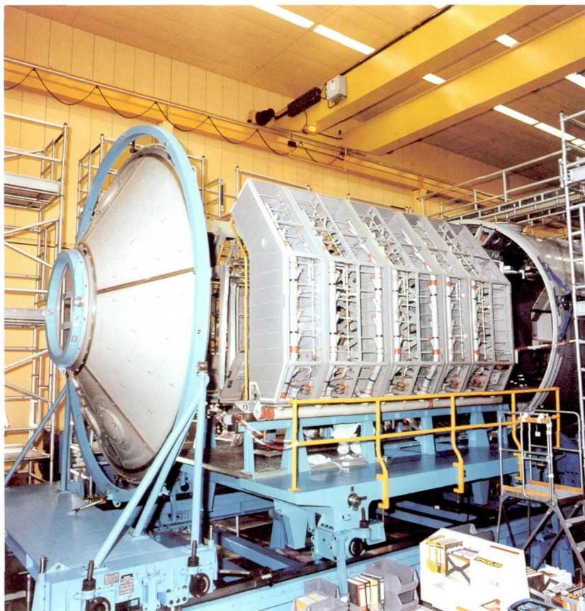
Figure 96. Experiment racks and aft end core ready for final assembly of the Flight Unit 1 module in the ERNO Integration Hall.
