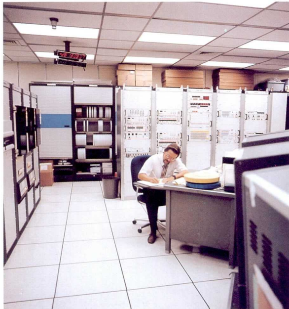
Figure 104. Electrical ground support equipment in the Spacelab control room at Kennedy Space Center.
