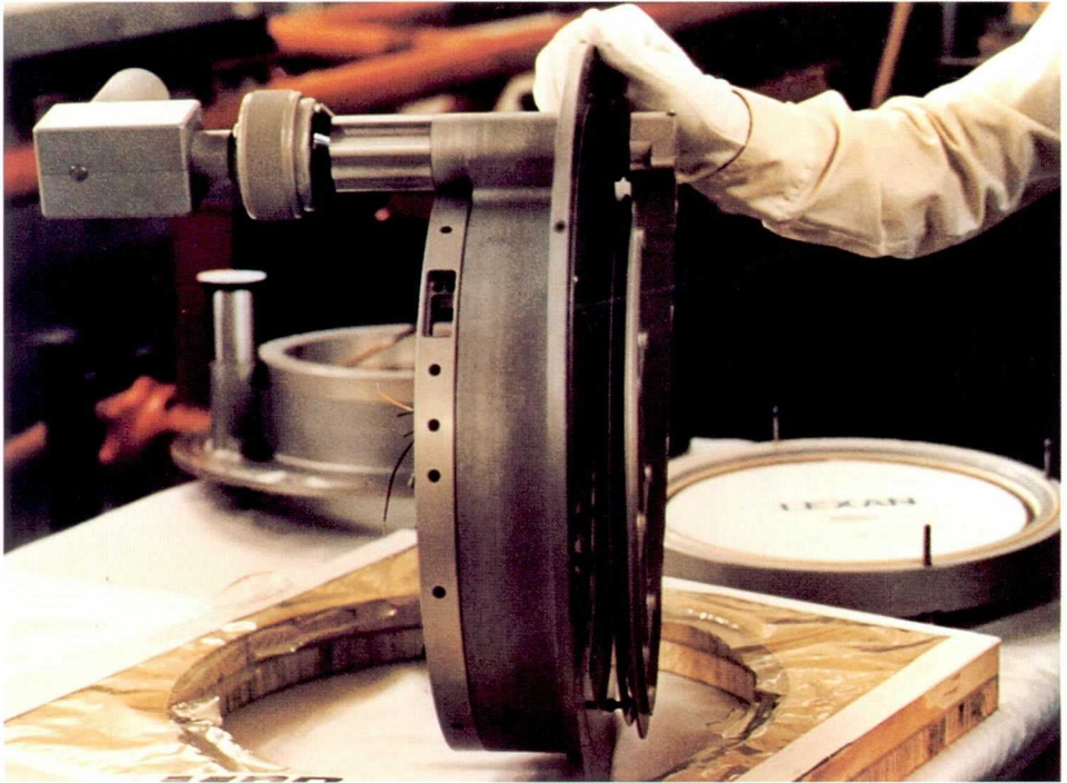
Figure 67. Engineering model viewport ready for installation in the top of the Spacelab module or in the aft end cone, 1980.
