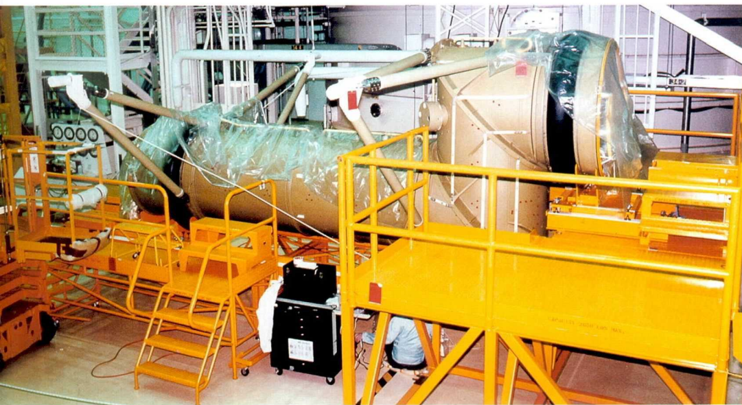
Figure 81. Transfer tunnel at Kennedy Space Center being readied for the Spacelab 1 mission.
