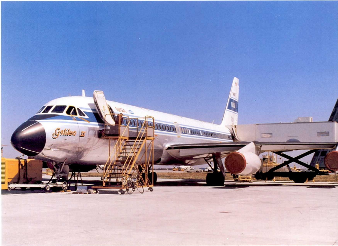
Figure 39. NASA's Convair 990 Galileo II with crew quarters in a lift van for times when the aircraft was parked between ASSESS flights.
