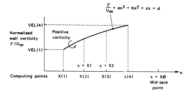
Normalised vertical velocity induced at XØ by the patch of vorticity extending from X1 to X2 is
