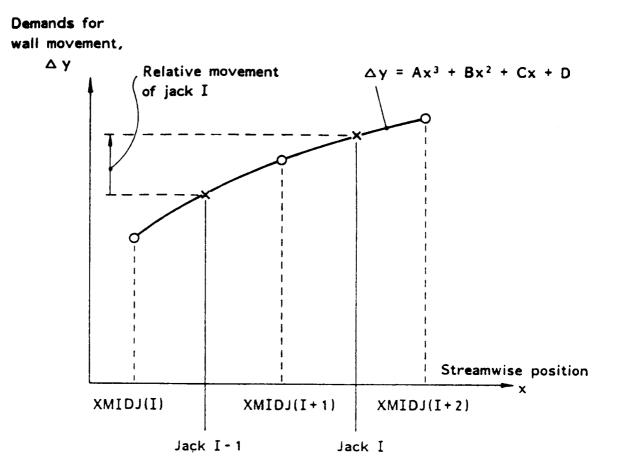
O Movements derived from integration of increments in wall slope.
